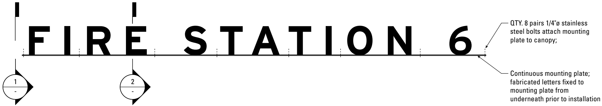
4 FRONT VIEW - BOLT LOCATIONS (APPROXIMATE) Scale: 1/4" = 1'-0"
