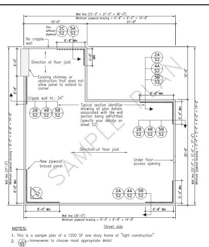
SAMPLE FOUNDATION AND PLYWOOD LAYOUT PLAN
