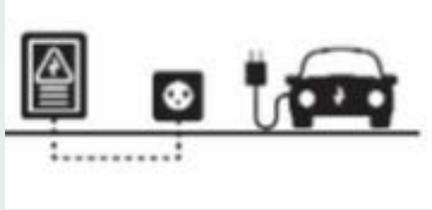
A diagram showing a power panel on the left connected by a dashed line to a car on the right. Between the panel and the car is a square icon with a lightning bolt and a plus sign, representing an overcurrent protection device. A charging cable is shown connected to the car. | EV Capable + overcurrent protection devices, wiring and outlet (i.e. full circuit)               |
