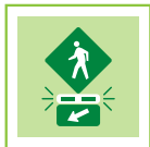
Rectangular Rapid Flashing Beacon
