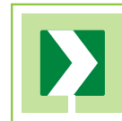
Chevron Signs on Horizontal Curves
