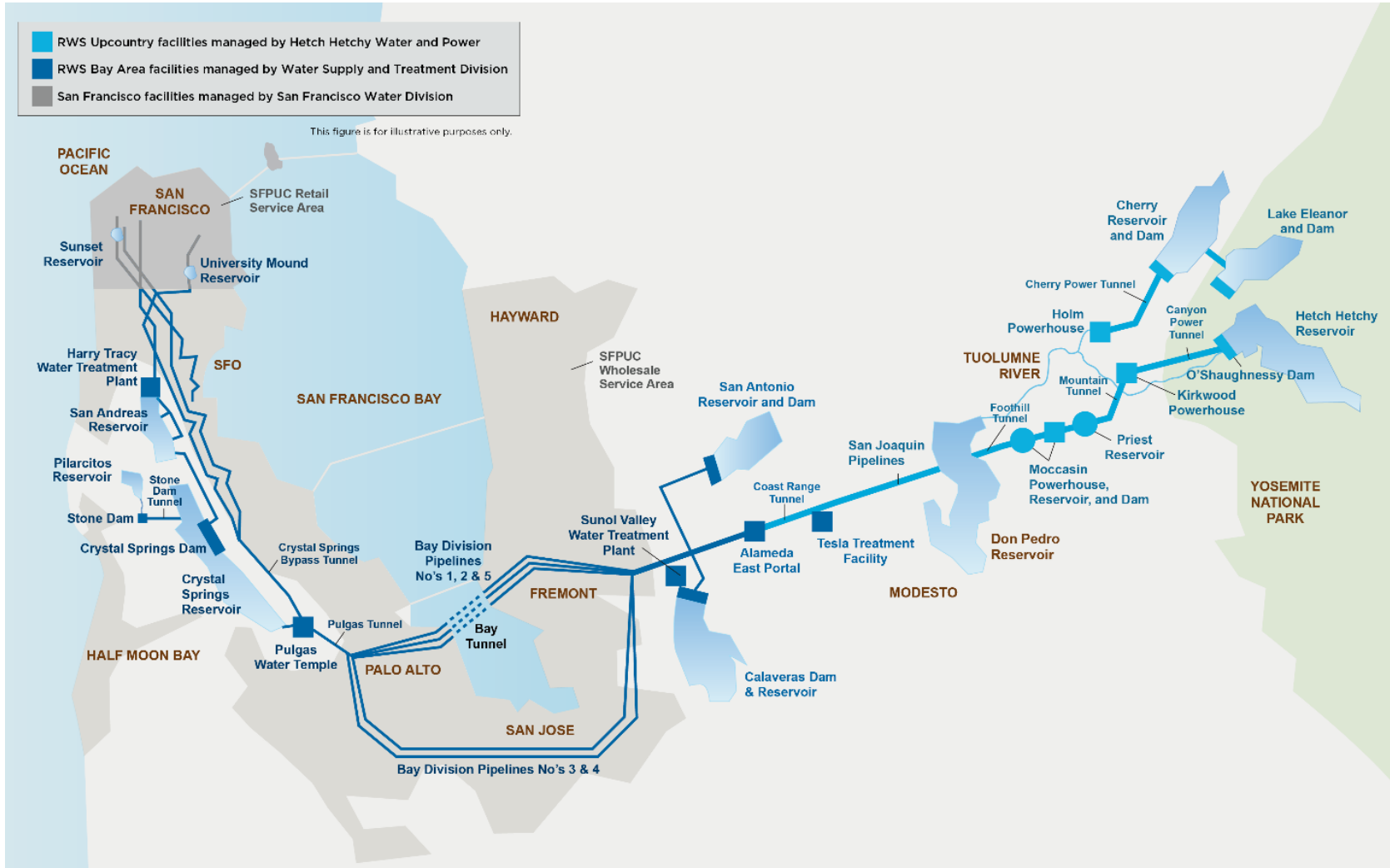
Figure 6-1. SFPUC's Regional Water System and Main Facilities
