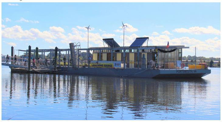
Floating Barge with wind and solar power
