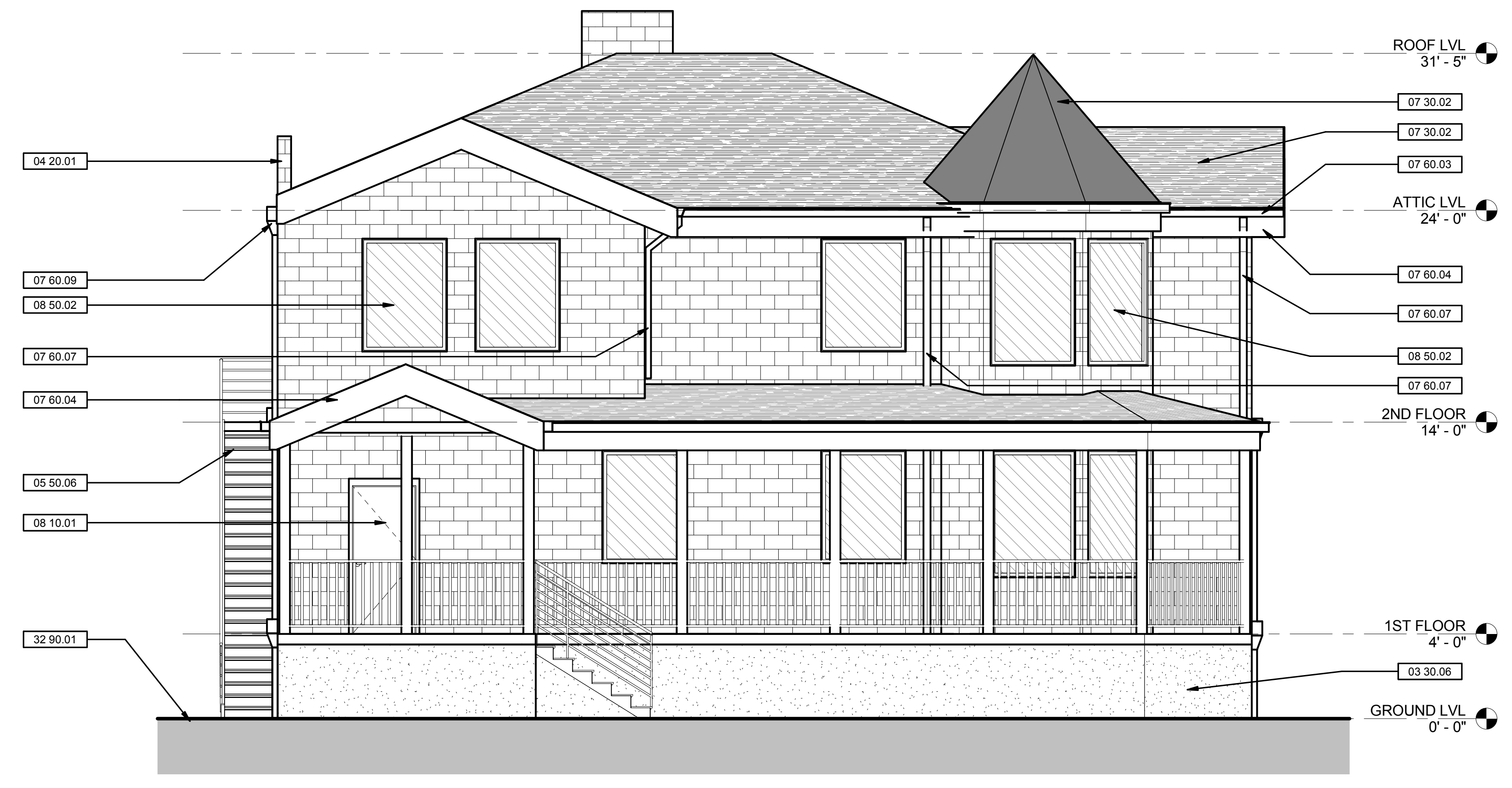
1 SOUTH EXTERIOR ELEVATION 1/4" = 1'-0"
