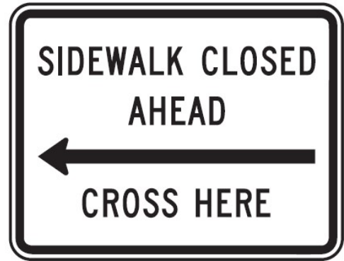
Figure 2. Sidewalk closed sign (R9-11, CA-MUTCD) should be used to show pedestrians where to cross when a sidewalk is closed.
