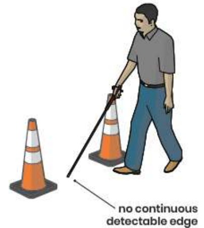
Figure 26. Traffic cones are not suitable channelization devices because they are not crashworthy and they do not provide a continuous detectable edge.
