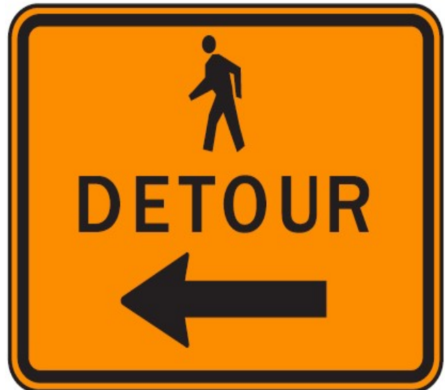
Figure 3. Pedestrian detour sign (M4-9b, CA-MUTCD) should be used to communicate when pedestrians should follow a detour route.
