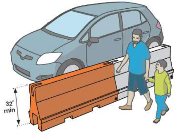
Figure 25. An example of a crashworthy channelization device which can be used to delineate a pedestrian or bicycle path.
